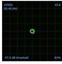
PHONO INTO LINE INPUT - Scratch Live is set to receive line level input. Set to the correct value in the setup menu.
