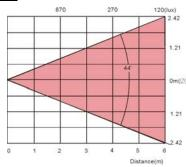
The Projector is best to be placed 5 meters from wall, and from this distance the light effect will cover an area of 4 m x 4 m.
