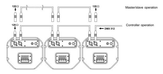
Only use a stereo shielded cable and 3-pin XLR-plugs and connectors in order to connect the controller with the fixture or one fixture with another.
