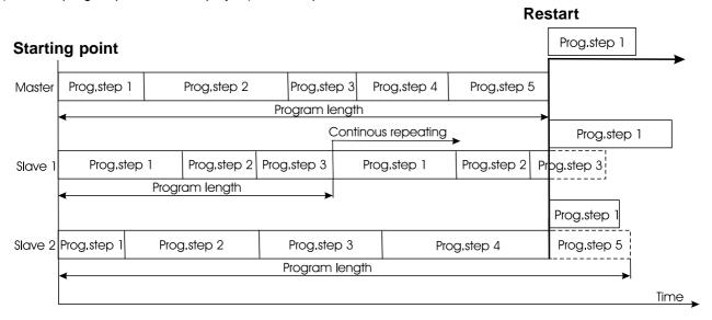
If the master fixture runs a reset, switches On/Off the lamp or plays test(program), all slaves will execute these acts too (e.g. if the master fixture has switched the lamp off, no slaves can switch the lamp on)! You can't play or edit any programs on the slaves by their control panels if the master is switched on and connected to the master/slave chain.
