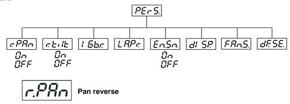
This function allows you to invert the pan movement. Use the **[Up]** and **[Down]** buttons to select **"On"** if you wish this feature or **"Off"** if you don't wish this feature and press **[Enter]** to confirm or **[Mode]** to cancel and return to the menu.
