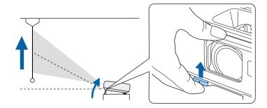
The foot extends from the projector. You can adjust the position up to 12 degrees.
