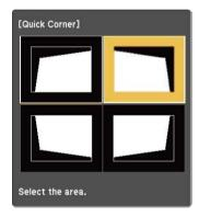
Press the arrow buttons to adjust the image shape as necessary. When you press [Enter], the Quick Corner adjustment screen is displayed.
