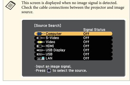
• Press the button for the source you want on the remote control. If there is more than one port for that source, press the button again to cycle through the sources.
