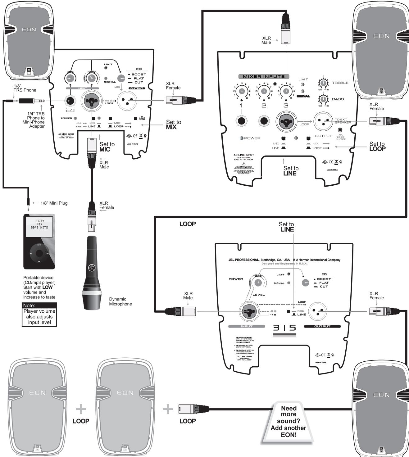
PA System With Powered Mains and Floor Monitors
