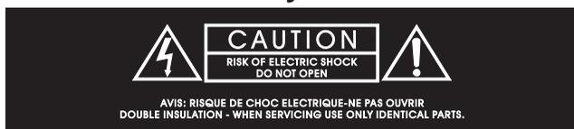
The lightning flash with arrowhead symbol within an equilateral triangle, is intended to alert the user to the presence of uninsulated. “Dangerous Voltage” within the products enclosure that may be of sufficient magnitude to constitute a risk of electric shock to
