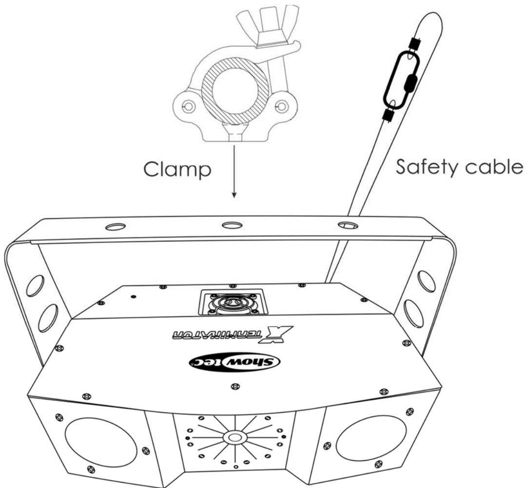
The X-Terminator can be placed on a flat stage floor or mounted to any kind of truss with a clamp.
