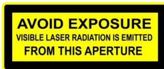
**CAUTION:** AVOID EXPOSURE TO BEAM: Avoid direct eye contact with laser light. Never intentionally expose your eyes or others to direct laser radiation.
