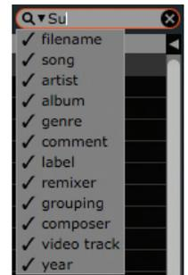
function will look through, click on the left hand side of the search box. The drop down menu shows which fields are currently being used. Press esc or the x button on the right of the search box to clear the search.
