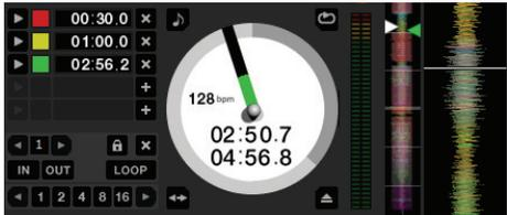
**TIP: Zoom in on the waveform using the – and + keys and ‘scrub’ to the desired position for greater accuracy when setting cue points.**
