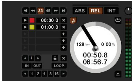
**REL** mode observes the relative forward and backward movement of the record, but does not take into account the position within the record. REL mode disables needle dropping, but allows skip-free scratching.
