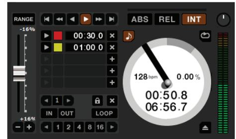
**INT** mode allows playing tracks without external vinyl (or CD) control. INT mode has a start / stop function and a virtual pitch slider. Holding down the shift key moves the pitch slider slowly. Holding the ctrl key and clicking on the pitch slider resets it to 33 RPM or 45 RPM, depending on which you are closest to at the time.
