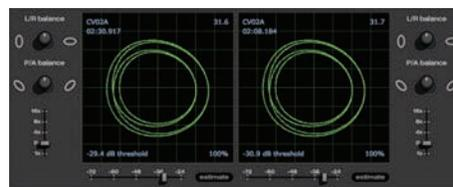
The scopes on the setup screen in Scratch Live display the input signal as a phase diagram. The key factors to look at on the scope display are crisp clean lines, round shape, and the tracking percentage in the lower right corner.
