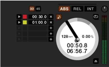
**ABS** mode is the default mode, and most closely resembles the properties of normal vinyl. The beginning of the track is mapped to the start of the record, and by picking up the tone arm and moving the needle to another part of the record (needle dropping) you can move to a different position within the track.
