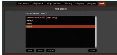
MIDI presets are accessible in the MIDI panel of the setup screen. By default, the current MIDI assignments in Scratch Live are automatically remembered and loaded next time you start the program. The preset screen allows you to save and recall several different MIDI setups. This is useful if you are using several MIDI devices or want to quickly switch MIDI setups without having to reassign all your controls.
