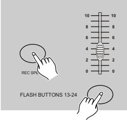
5. While pressing and holding down the Rec Speed button, tap the Flash button(13-24) that stores the program.
