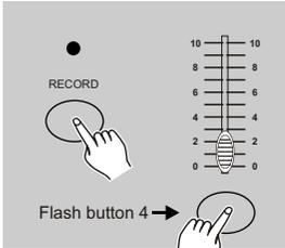
Tap the Flash button 4 three times while holding down the Record button, the Segment Display reads "OUT" indicating the controller is ready to send a file.
