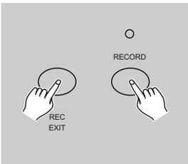
5. Tap the Rec Exit button while pressing and holding down the Record button, the Scene LED goes out, indicating the exit of Edit mode.
