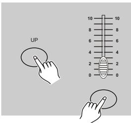
4. While holding down the Up or Down button, tap the Flash button corresponding to the DMX channel of the scene you wish to modify until you reach the desired intensity value read from the Segment Display. Then you may tap the Flash buttons until you are satisfied with the new scene.
