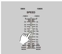
4. Move the Speed slider until the Segment Display reads your desired value.
