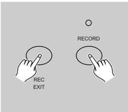
Press and hold down the Record button. While holding down the Record button tap the Rec Exit button to exit MIDI setting.
