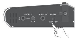
Turn on the power in the order of source devices → output devices.
