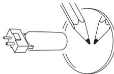
To minimize the risk of gobo overheating and damage, install a coated gobo with the more reflective side facing towards the lamp.
