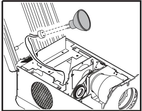
5. If you touched the bulb, the reflector or any optical components, clean them with a clean, lint-free cloth wetted with isopropyl alcohol. Alcohol is extremely inflammable, so take precautions to avoid fire risk.
