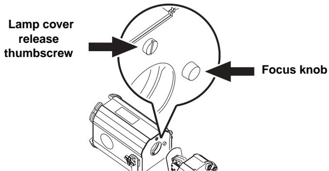
3. Remove the old lamp and socket from the lampholder and, being careful not to strain any wires, gently pull the lamp off its ceramic socket.
