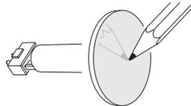
The less reflective side of a coated gobo will absorb less heat if it faces away from the lamp.
