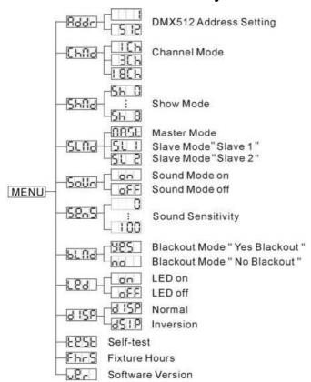
System Menu: When making adjustments press ENTER to confirm your setup and then press and hold the MENU button for at least 3 seconds. To exit without making any adjustments press the MENU button.
