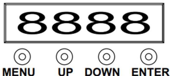
1~Press MENU Can circulate 8 different functions. The front 2Digits mean the function it has. (Please see the function form as follow.) And the last 2Digits mean the function's address, speed or parameter. Press UP or DOWN can change the value. And press ENTER to confirm.
